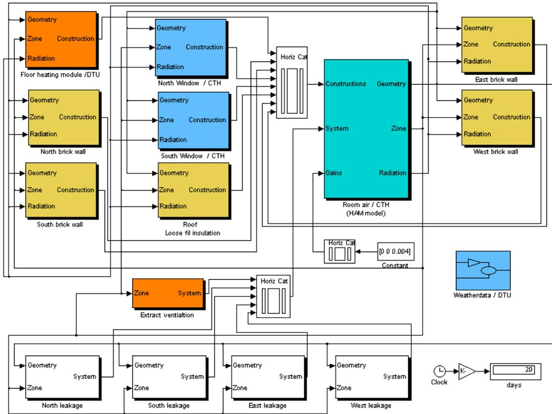
Figure 4. Simulink model of the house from Figure 1.
