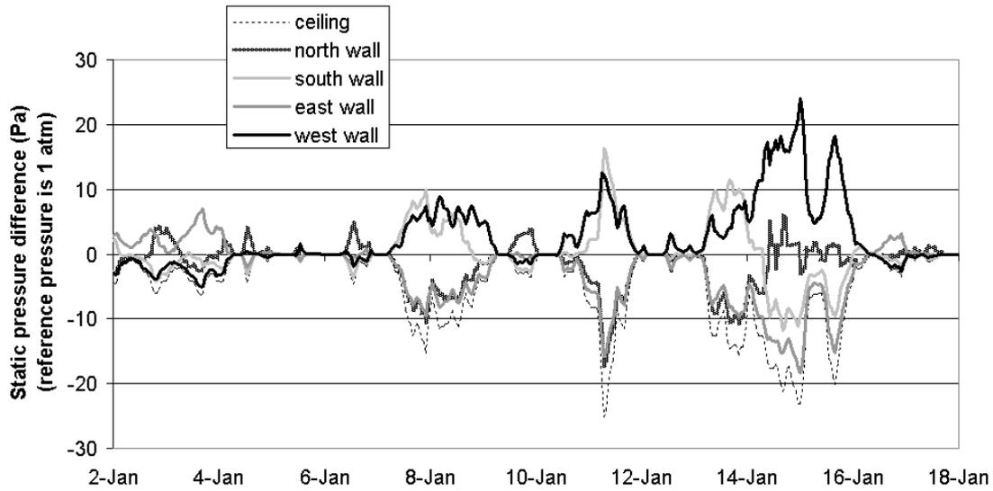
Figure 5. Static pressure difference (against the reference pressure) at each of the surfaces.
