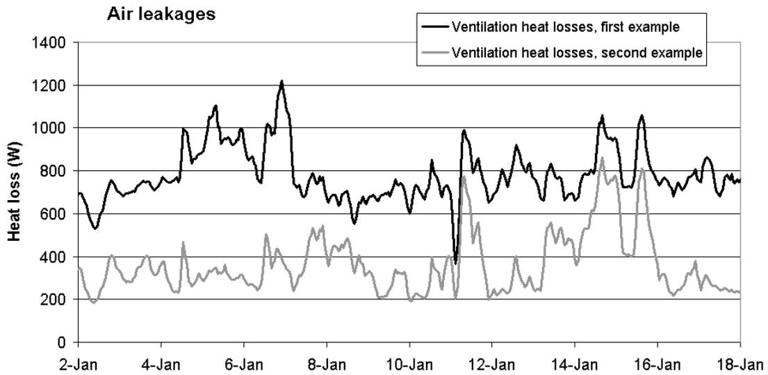
Figure 9. Ventilation heat losses through leakages. Indoor air temperature is the reference one.
