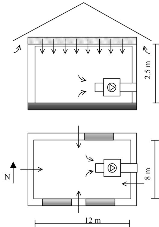
Figure 1. Section and plan of the house. Airflow paths are indicated with arrows.
