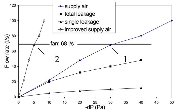
Figure 3. Flow characteristics for the supply air and air leakage paths.
