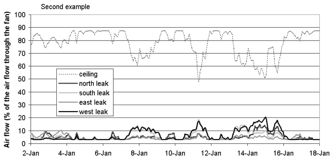
Figure 7. Results for the second example. Air flows through indicated openings
