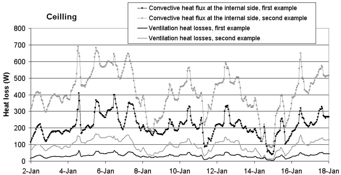
Figure 10 Heat losses through the ceiling. Indoor air temperature is the reference one.
