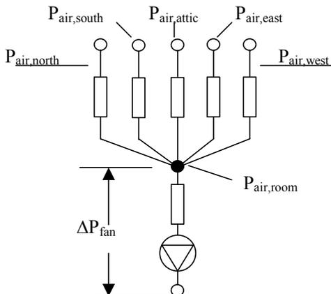
Figure 2. Air pressure drop model of the house
